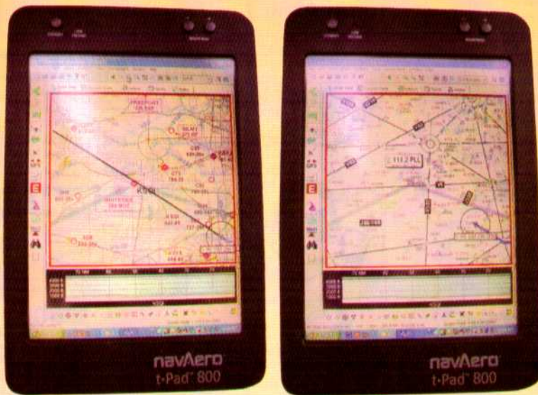
LEFT: The t-Pad 800 did a good job of displaying Jeppesen's FlightMap software, which we used to change course using the leader line to reach our destination. RIGHT: The t-Pad 800 can show both VFR and IFR maps, and even approach plates with the right software package, providing full electronic flight bag capabilities in the cockpit.
